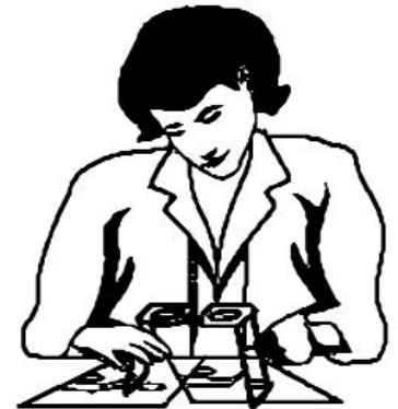
Figure 3.2. Using the pocket stereoscope. The stereoscope is aligned horizontally and centered along the seam separating the image pairs.
